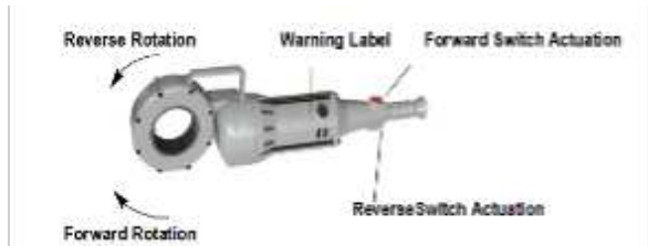
Figure 3 – Switch Position for Rotational Direction
