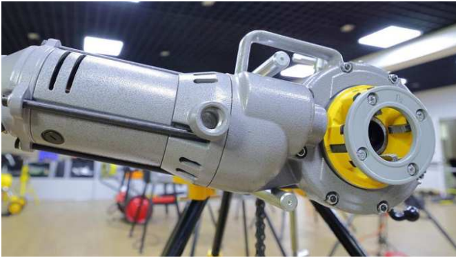
Figure 4 – Installing Die Heads into PD7 Power Drive
