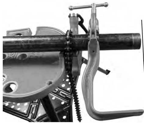
Figure 5 – Support Arm Aligned with End of Pipe
