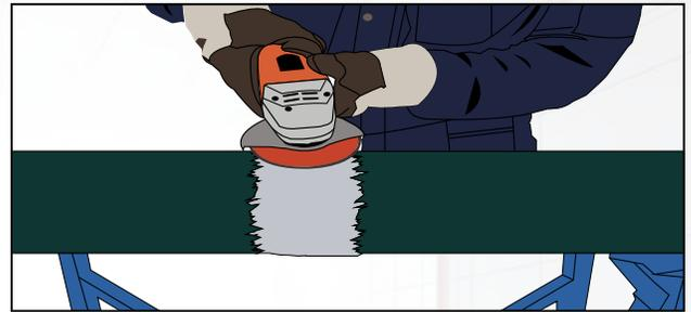
Figure 3.b. Initial Grinding.
