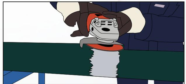
Figure 3.f. Grind surface.
