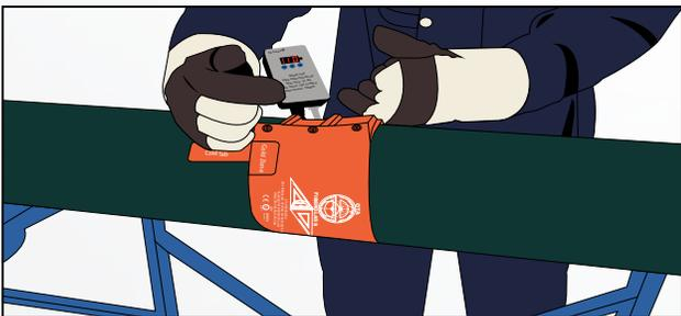
Figure 3.e. Apply Heating Blanket Constant Temp.
