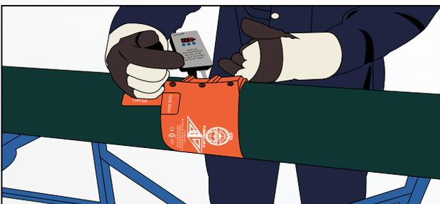
Figure 3.e. Apply Heating Blanket Constant Temp.
