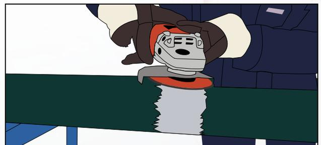
Figure 3.f. Grind surface.
