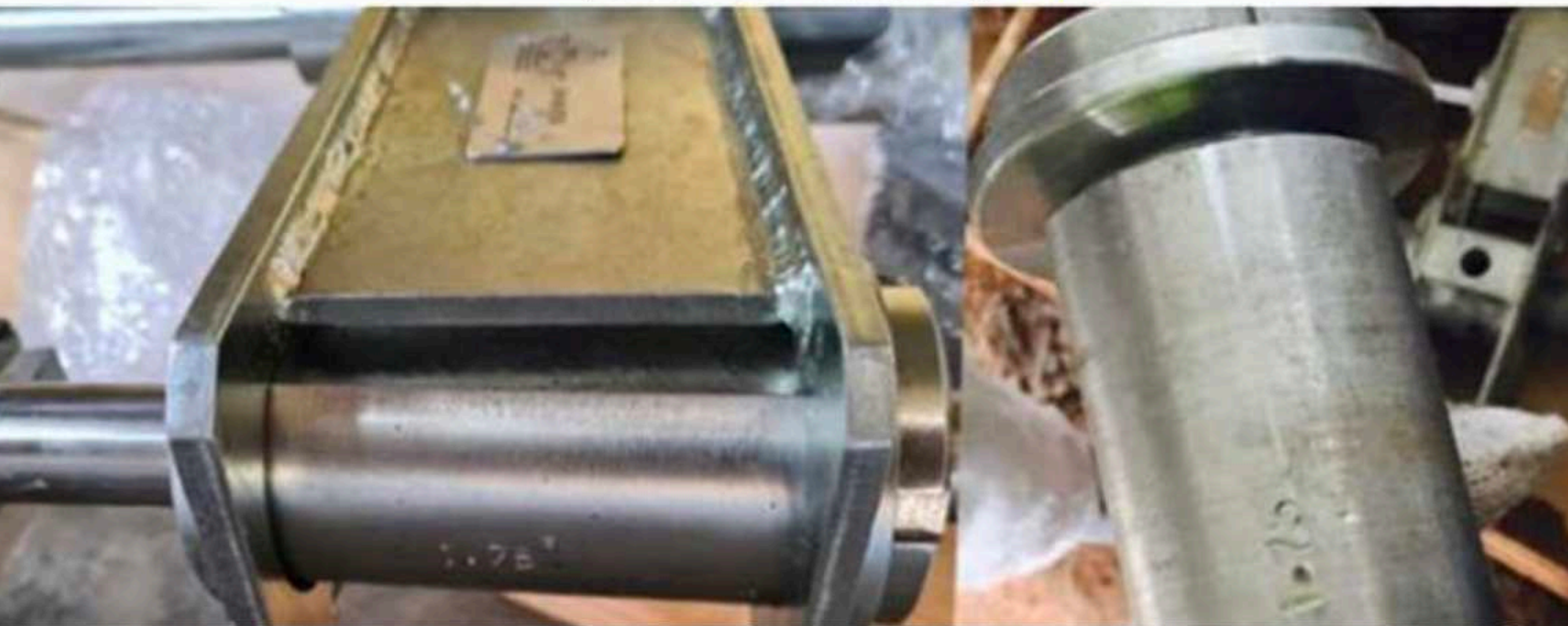
Pipe Shaver With Standard Taper Angle - 1.75^\circ
